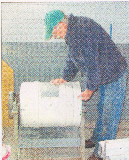
David Tait demonstrates how the tumbler, used to break up the dry clay, works.
