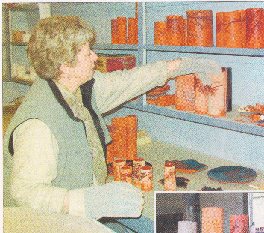
Judy Tait arranges pieces of pottery taken straight from the kiln. The inset photo shows examples of pieces that are (from left to right) unfired, bisque-fired (fired once), and fired twice. The color intensifies with each firing as the iron oxidizes in the high heat.
