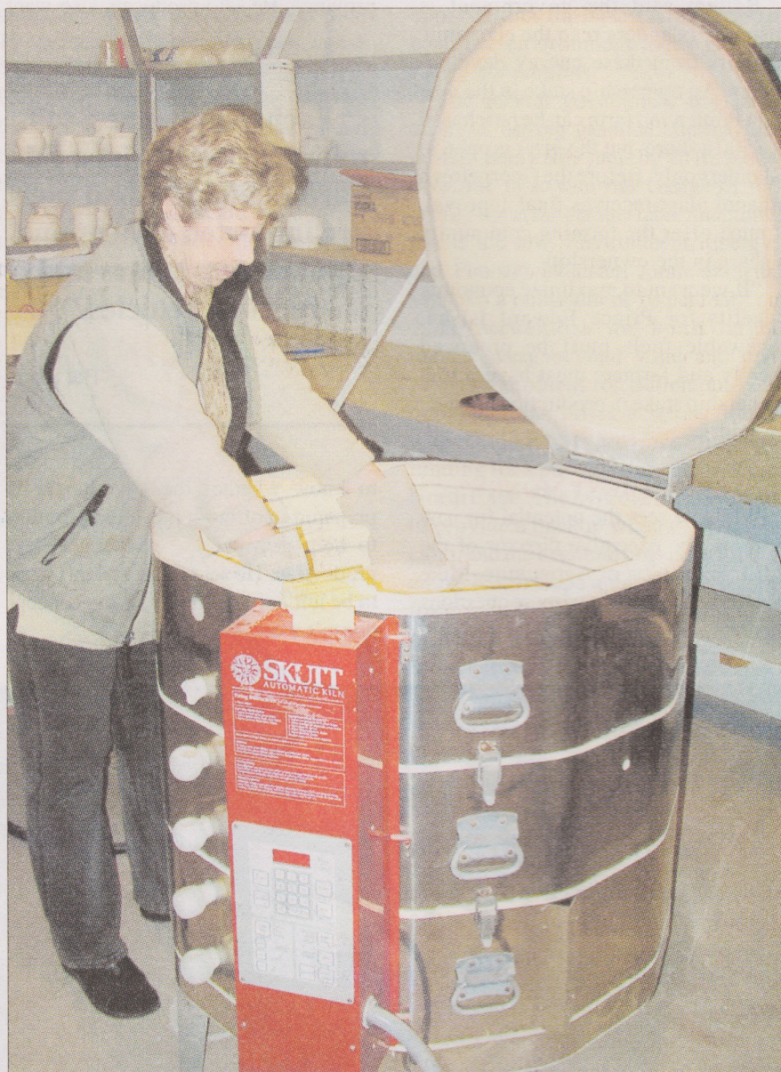
Judy Tait removes pottery from the kiln. The kiln reaches temperatures of 2000 degrees Fahrenheit and it was trial and error in finding a clay that worked for them.
